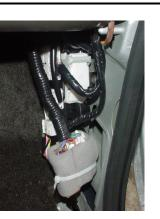
Without AMP: Secure to lower bracket opening.
